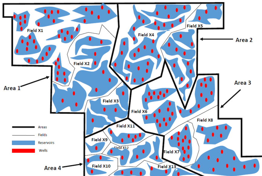
Figure 2. Schematic diagram of Block K (Angola) showing the areas, fields, reservoirs and wells. See Table 1 for detailed breakdown of the distribution of the areas, fields, reservoirs and wells for the Block K.
