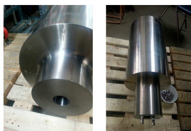
Figure 9. CEDM nozzle specimen with a J-groove weld.
