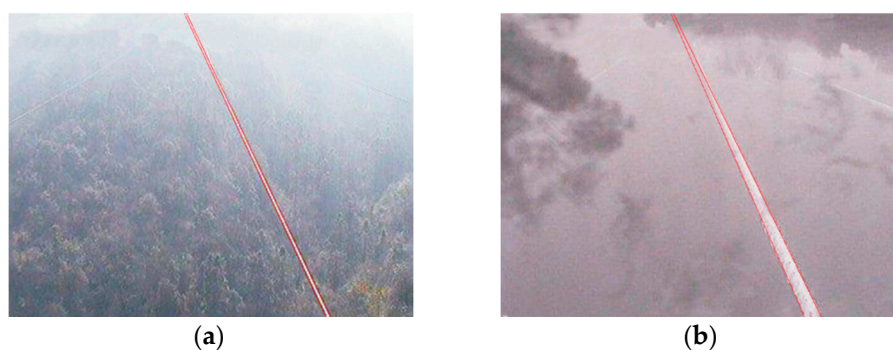
Figure 15. Accurate positioning results are placed into the original color images. (a) Accurate positioning result of an un-iced power transmission line; (b) Accurate positioning result of an iced power transmission line.
