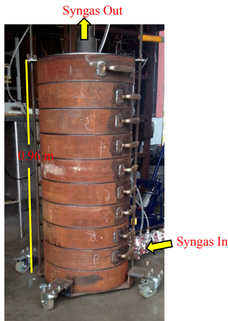
Figure 3. 10-layered biomass-based filter system.
