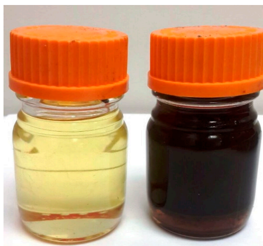
Figure 8. Canola oil (used in oil bubbler for treatment III) before and after the test.
