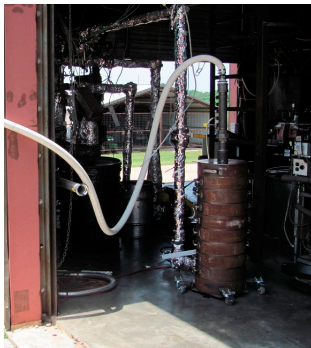
Figure 2. Wood shavings filter column installed with a gasifier system at Oklahoma State University.
