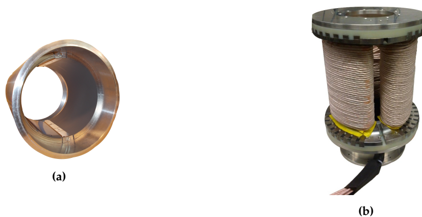
Figure 3. Photographs of rotor and stator of SRM prototype. (a) The assembled outer-rotor prototype, not including the central shaft. One half ferromagnetic and one half austenitic stainless steel; and (b) the three-phase stator with windings. The aluminum lid is on top, with a plastic plate separating it from the standing laminated c-shaped bits. The windings are wound around each of the three groups of c-shaped bits. The stator is hollow to allow for a shaft in the prototype.
