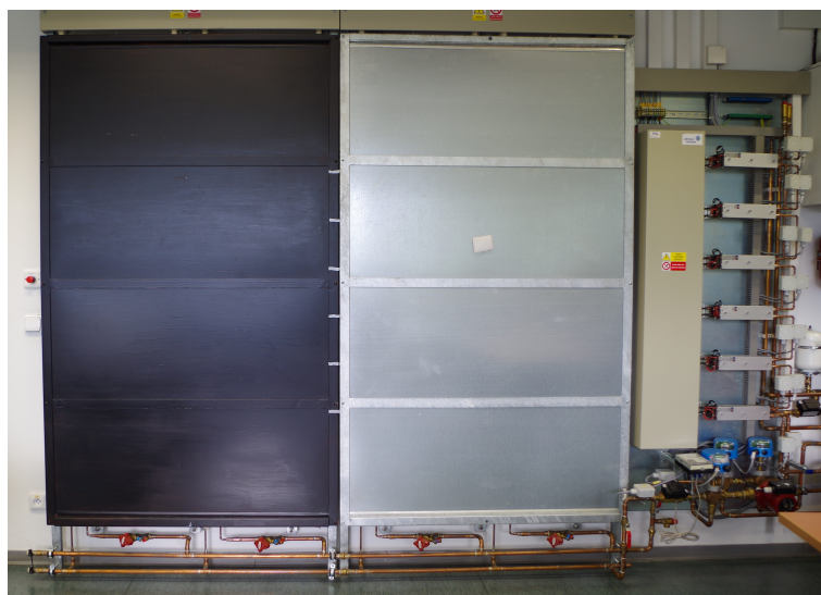
Figure 10. Thermal panels with the original and modified surfaces.
