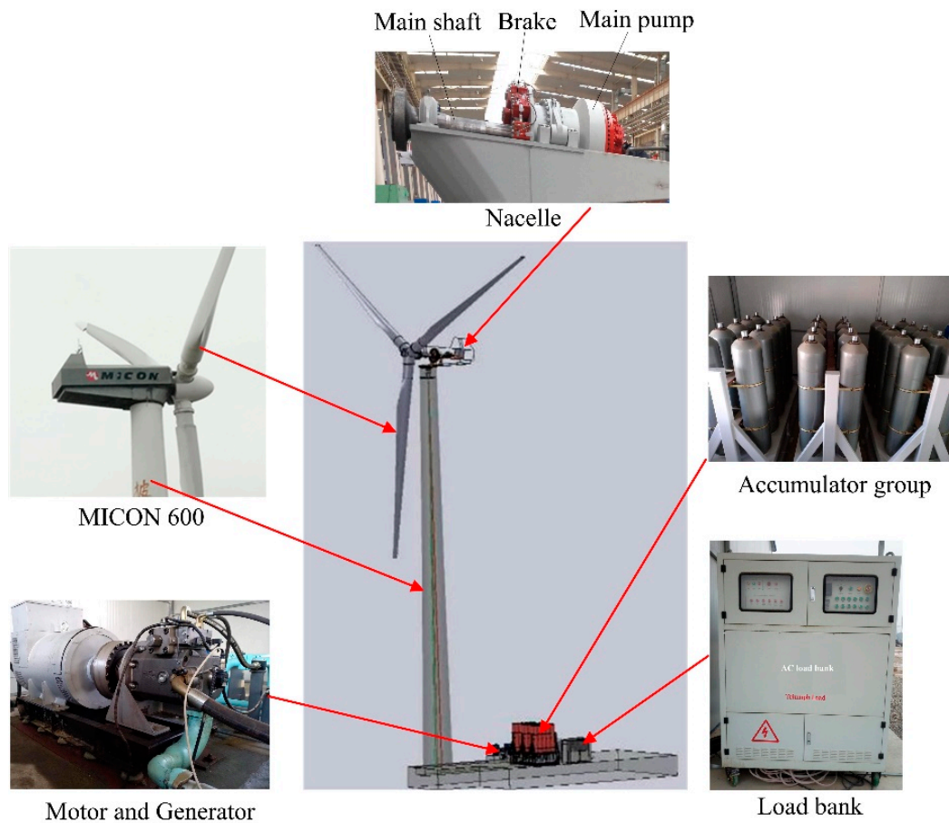
Figure 11. The layout design of 600 kW hydraulic energy storage wind turbine test rig.
