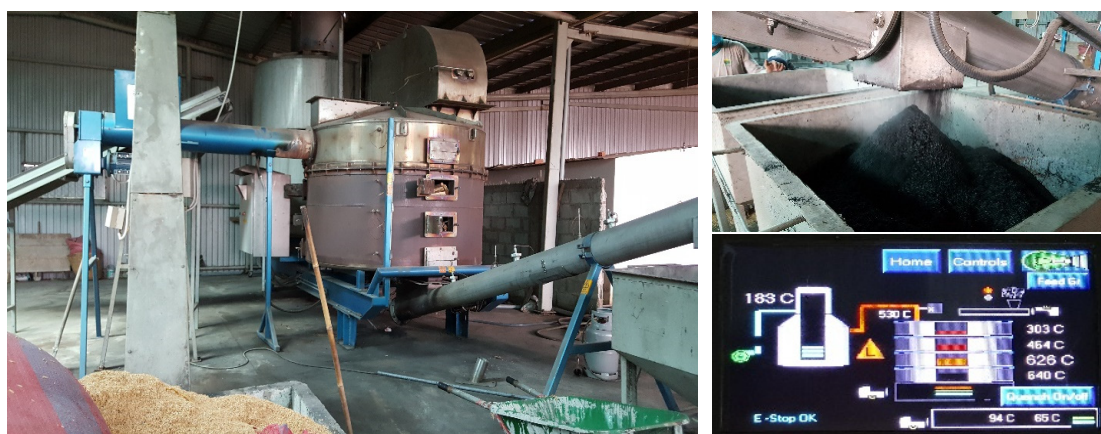
Figure 1. Full-scale gasification system (BiGchar 2200 fast rotary hearth, Pyrocal Pty Ltd, Wellcamp, Queensland, Australia) for biochar production. Owned by Ecofarm Co. Ltd., Long An province, Vietnam.
