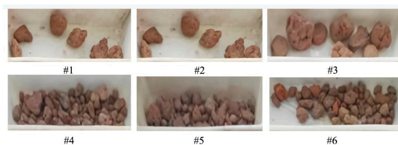
Figure 5. Clinker with various particle sizes in the different batches.
