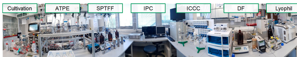
Figure 2. Laboratory set-up of the continuous production of a monoclonal antibody. ATPE (aqueous two-phase extraction), SPTFF (single-pass tangential flow filtration), IPC (interprocess communication), iCCC (integrated counter-current chromatography), DF (diafiltration), Lyophil (lyophilization).
