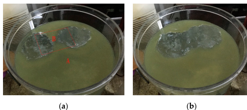
Figure 8. The slag eyes in the water model with double porous plugs (16 mm OLT): (a) Q = 0.286 \text{ m}^3/\text{h} , (b) Q = 0.381 \text{ m}^3/\text{h} .
