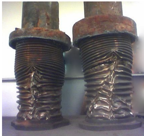
Figure 1. Effects of water hammer dynamics. (Cited from: https://en.wikipedia.org/wiki/Water_hammer ).
