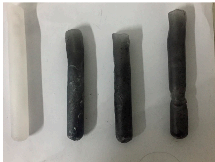
Figure 6. The comparison of dispersion stability of CPCM. Left to right: pure paraffin, 2% EG/paraffin, 2% GO/paraffin, 2% GR/paraffin.
