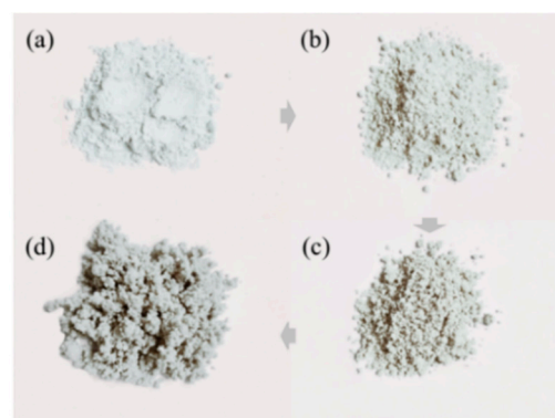
Figure 5. Wet montmorillonite particles with water ( w ) contents of (a) 15%, (b) 20%, (c) 30% and (d) 40%.
