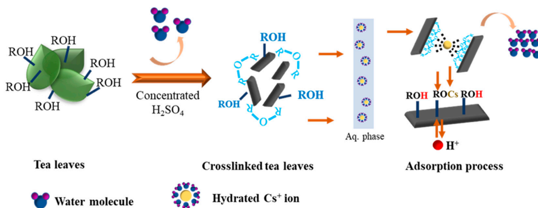
Scheme 1. Modification of tea leaves and Cs adsorption process in the aqueous phase.
