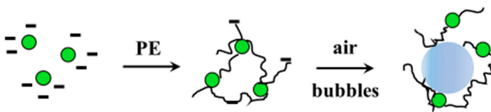
Figure 2. Charge neutralization effects of a hydrophobic cationic PE, followed by its binding to air bubbles.
