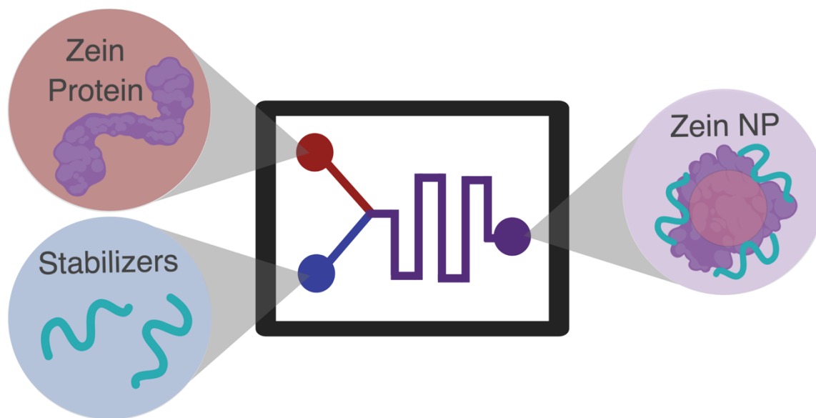
Figure 1. A graphical depiction of the Zein nanoparticle (NP) synthesis using a coprecipitation microfluidics system. At the inlet channels, the organic phase is indicated in red while the aqueous phase is blue.
