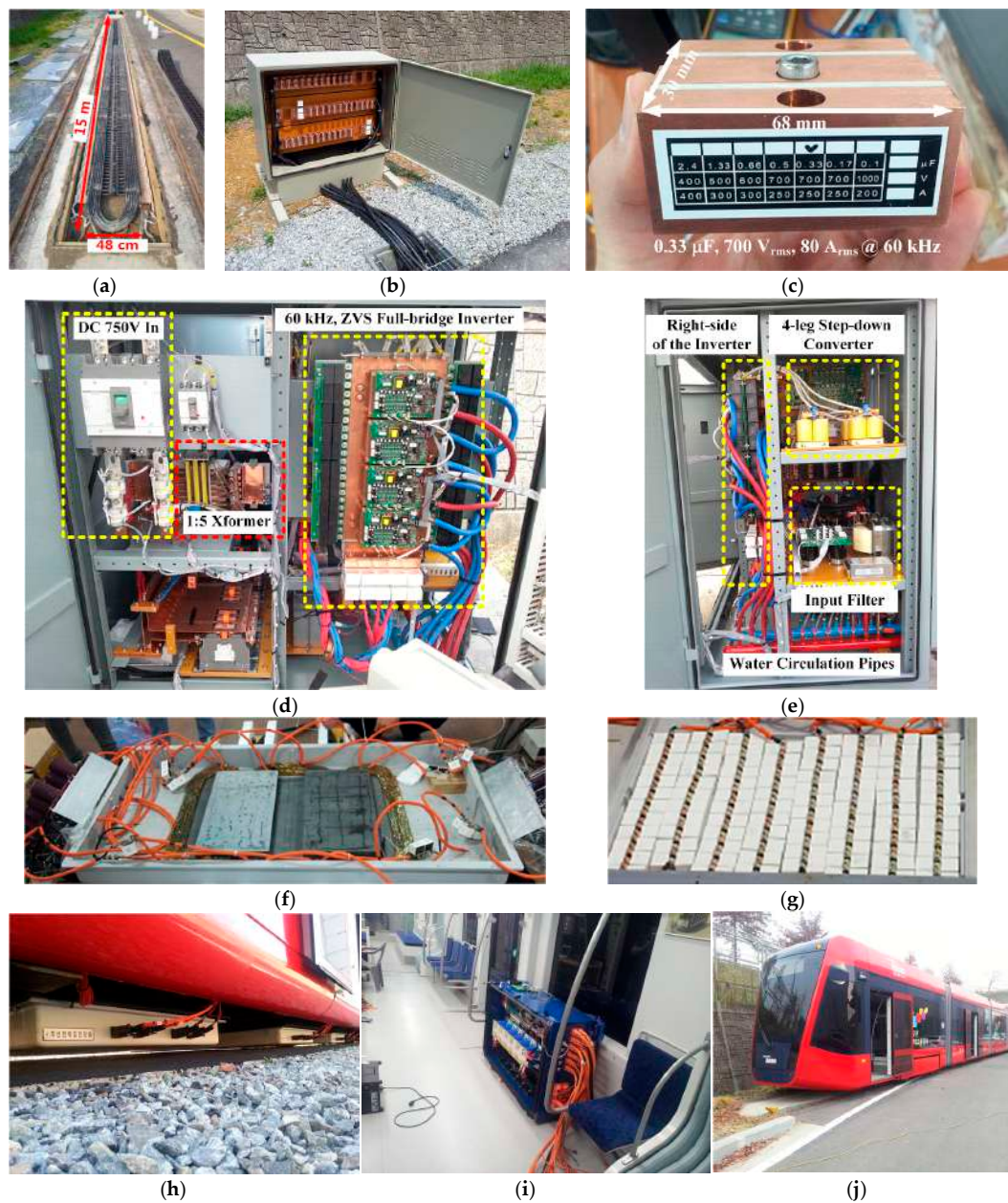
Figure 10. Photographs of the developed test-bed: (a) transmitter; (b) transmitter tuning capacitor bank; (c) transmitter tuning capacitor; (d) the PAM inverter; (e) interleaved DC-DC converter; (f) pick-up winding; (g) pick-up tuning capacitors; (h) installed three pick-ups; (i) pick-up output voltage regulator; and (j) target tram.
