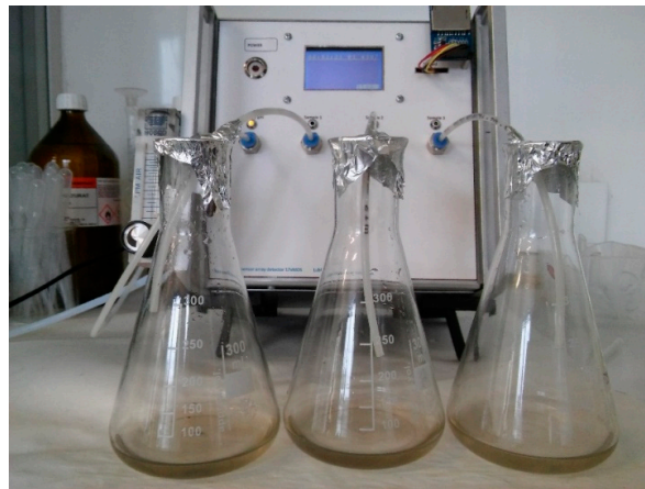
Figure 2. Analysis of wastewater samples by means of a gas sensor array.
