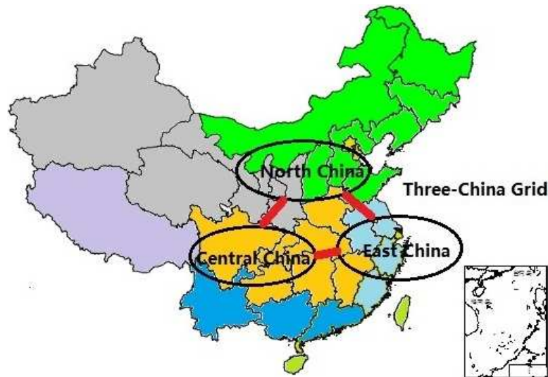
Figure 1. Diagram of the Three-China synchronous 1000 kV grid.
