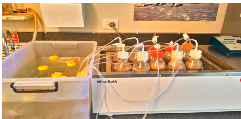
Figure 2. Bagasse fermentation and collection of CO 2 gas equipment.
