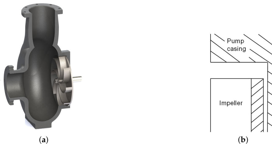
Figure 2. (a) Vortex pump according to the covered design; and (b) schematic illustration of the covered design.
