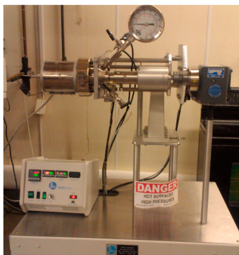
Figure 1. Stirred Parr reactor operating in horizontal position.
