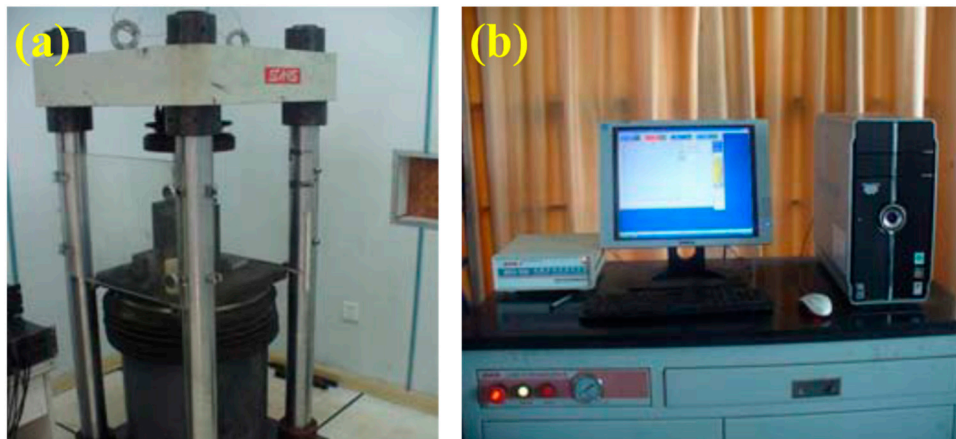
Figure 3. Axial compressive loading subsystem. (a) Loading frame. (b) Hydraulic drive device and controller host.
