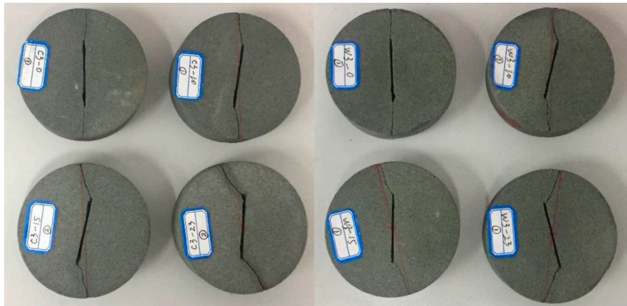
Figure 3. Failure modes of some sandstone specimens.
