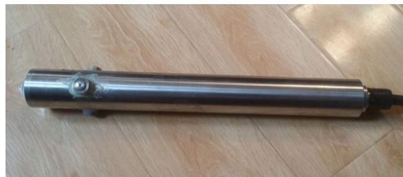
(a) The MA15Z mine-specialized coal stress meter.
