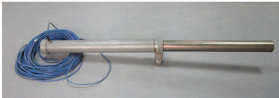
(b) The MA650 mine-specialized roof displacement meter.
