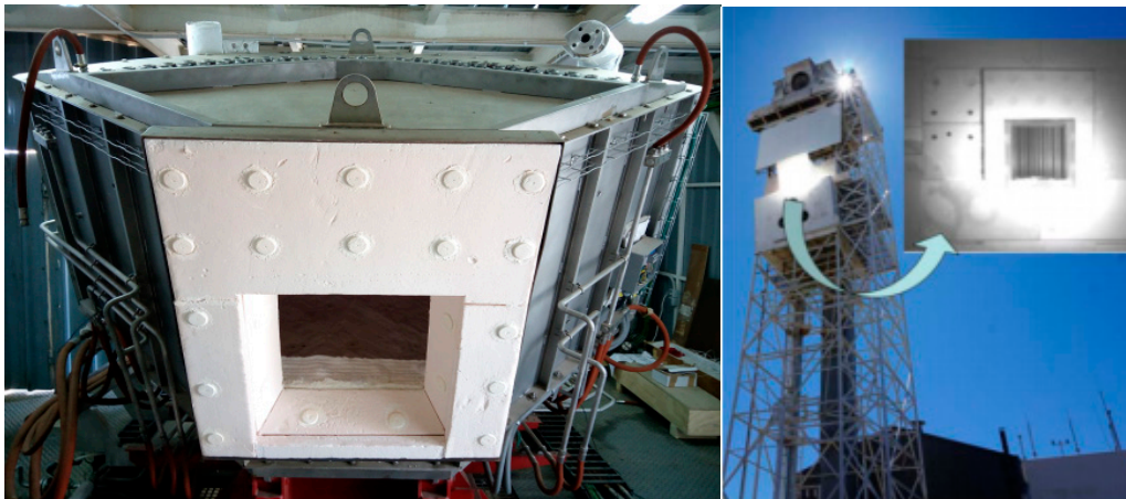
Figure 4. (left) Frontal view of the reactor installed in CRS (Central Receiver Solar) tower plant; (right) View of the reactor being irradiated by CRS field.
