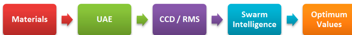
Figure 1. General scheme of the solution approach in this study. UAE: ultrasonic-assisted extraction; CCD: central composite design; RMS: Response surface methodology.
