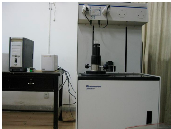
Figure 1. MK-AutoPore IV9510 mercury injection apparatus.
