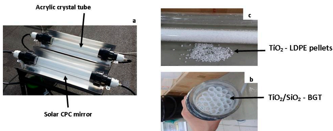
Figure 1. Photoreactor: (a) solar compound parabolic collector (CPC) reactor; (b) \text{TiO}_2/\text{SiO}_2 -borosilicate glass tubes (BGT); and (c) \text{TiO}_2 -low density polyethylene (LDPE) pellets.
