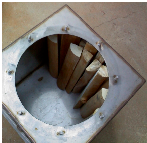
Figure 2. Loading the carbonization chamber with dried wood pieces.
