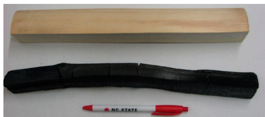
Figure 4. Comparison of oven-dried yellow poplar biomass ( top ) to the charcoal produced ( bottom ).
