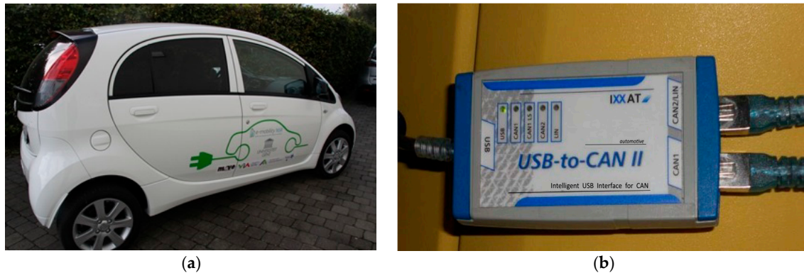
Figure 1. (a) Electric vehicle (EV) shared by the co-housing community during the e-Mobility project [57]; and (b) equipment for the Controller Area Network bus (CAN bus) data acquiring.
