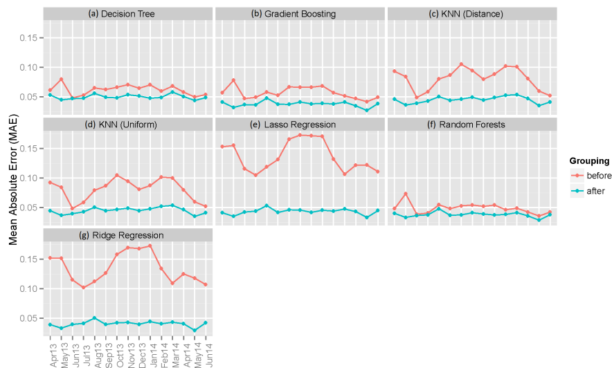
Figure 6. Average MAE values of seven individual machine learning models' point forecasts before and after grouping of data by hours of the day. Results for: (a) decision tree; (b) gradient boosting; (c) KNN (distance); (d) KNN (uniform); (e) lasso regression; (f) random forests; and (g) ridge regression.
