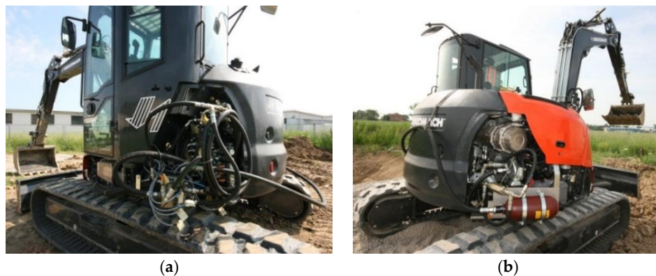
Figure 6. View of two sides of the instrumented hybrid excavator: (a) HCV; and (b) accumulator.
