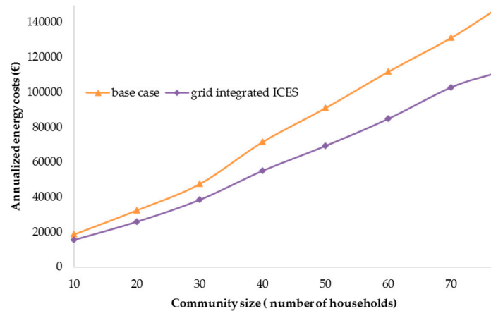
Figure 9. The effect of community size on total energy costs of the ICES.
