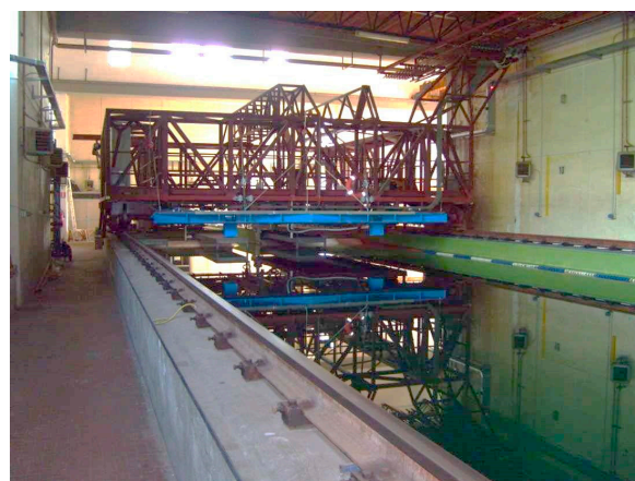
Figure 3. Towing tank and towing carriage.
