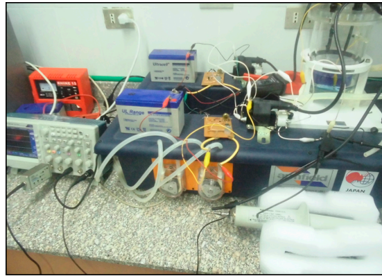
Figure 2. Plasma treatment system using corona discharge.
