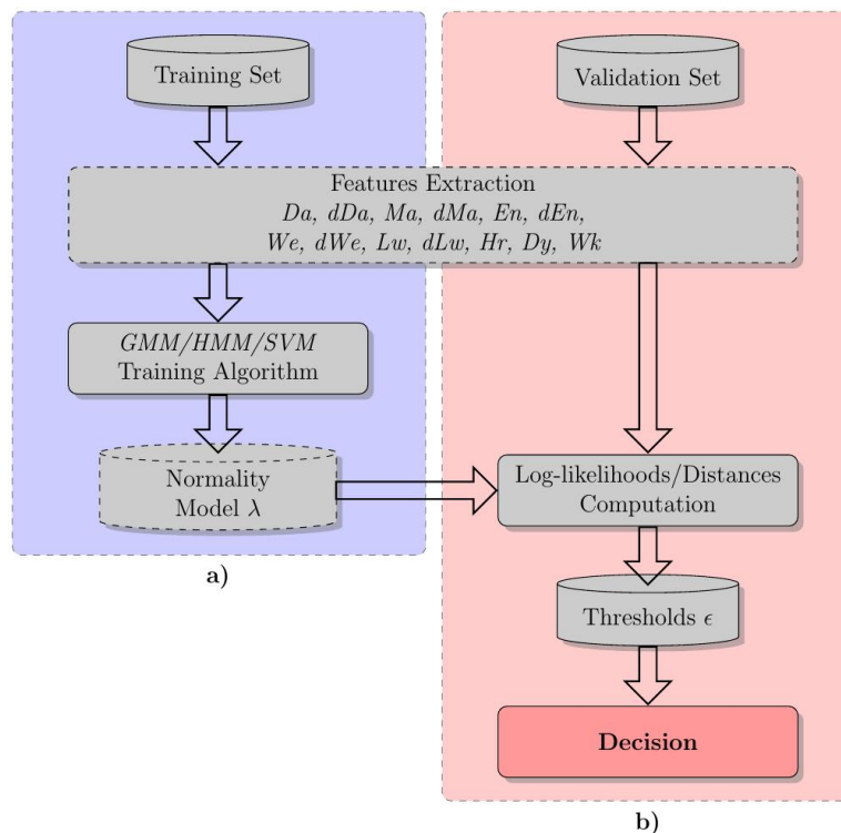
Figure 1. Framework stages: (a) normality model creation; (b) novelty detection.
