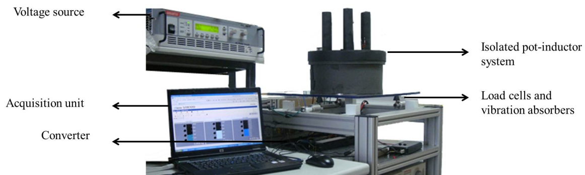
Figure 9. Test-bench for efficiency evaluation with labeled main components.
