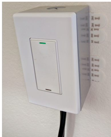
Figure 5. A ZigBee light switch is used to control devices and provide user feedback.
