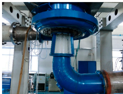
Figure 2. The pump-turbine model.
