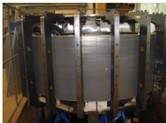
Figure 5. A direct driven three phase 225 kW permanent magnet synchronous cable wound generator.
