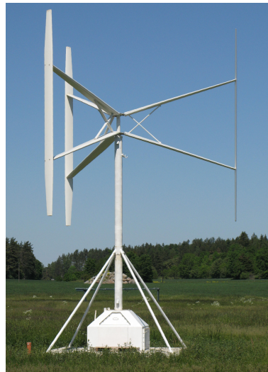
Figure 7. Three bladed 12 kW prototype vertical axis wind turbine located north of Uppsala.
