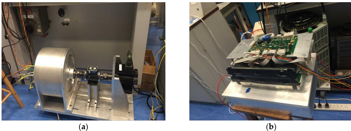
Figure 5. Prototype of the DSFM motor and its controller: (a) test machine; and (b) back-to-back controller.
