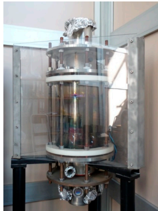
Figure 5. The PROTO-PINCH vacuum vessel.
