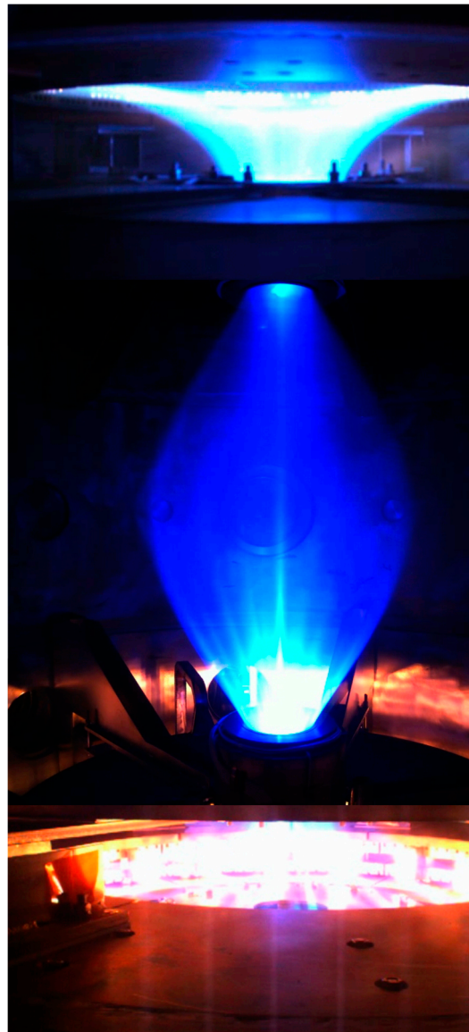
Figure 17. Comprehensive representation of the PROTO-SPHERA plasma center post, obtained by merging three images captured during a typical experiment by high resolution cameras.
