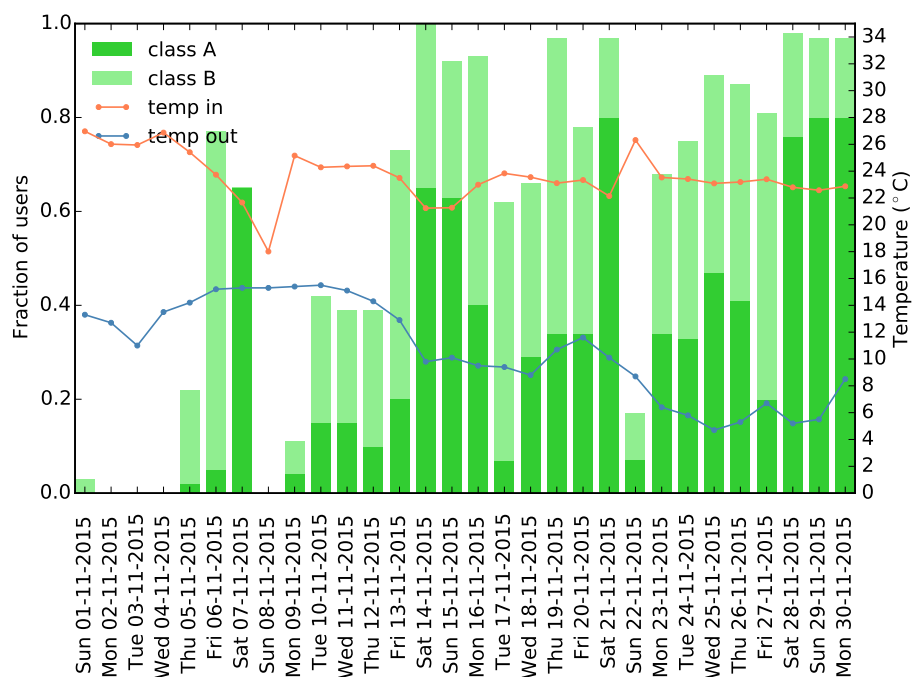
Figure 5. Comfort analysis w.r.t. ISO 7730/2005 November 2015, comfort classes daily percentage plotted on the main vertical axis.
