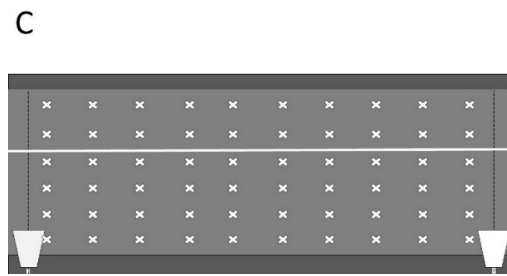
Figure 1. Locations of luminaires (white cones) and points (white x) for average road surface luminance and luminance uniformity measurements. (A) Road with two lanes with painted road markings; (B) road with two non-separated lanes; and (C) pedestrian and bicycle road. Dotted lines show the start and end of the measurement area. Darker areas are outside the road surface. The diagrams are sketches, not scale drawings.
