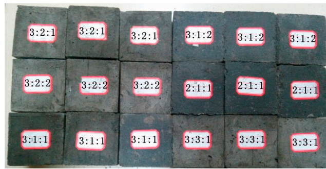
Figure 6. Photograph of 7 cm cubes of coal seam simulation material. The numbers on the cubes represent the different coal: cement; gypsum ratios used to manufacture the test cubes.
