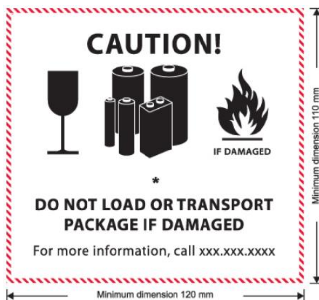
Figure 1. Labeling required for packages containing lithium-ion batteries or products with installed lithium-ion batteries to be shipped by air [2]. Reproduced with permission of the United Nations (UN).
