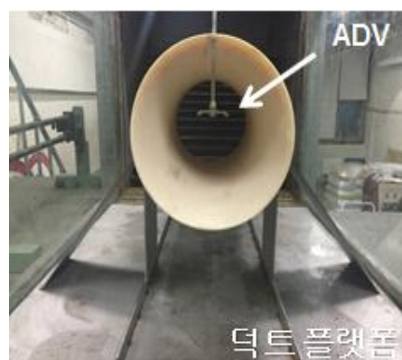
Figure 8. Installed duct mock-up.
