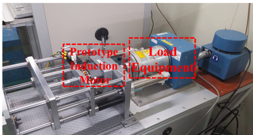
Figure 11. Experimental dynamometer setup for the test of prototype.
