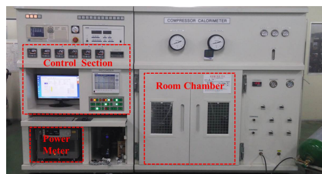
Figure 15. Experimental calorimeter for the test of prototype.
