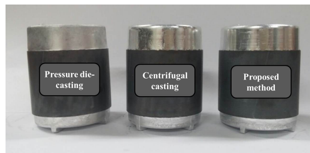
Figure 7. Prototype rotors according to the casting method.
