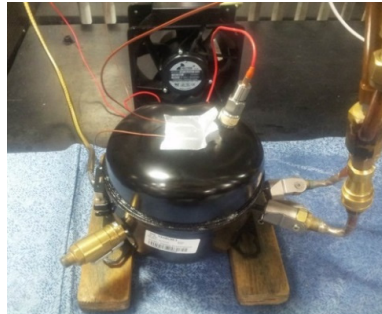
Figure 14. A single-phase hermetic reciprocating compressor.
